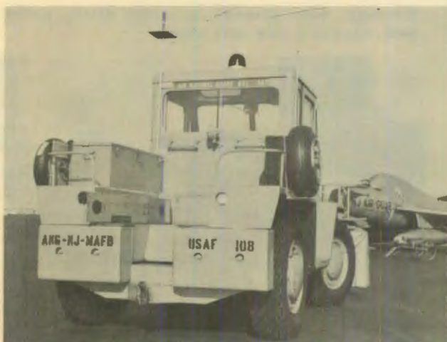
Rear view of the Coleman showing the ramp, additional spare wheels, tool kit, and radio installation.
